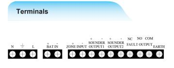
N, L: 220VAC power terminals BAT IN (+, -): Battery terminals ZONE INPUT (+, -): Loop terminals. SOUNDER OUTPUT1 (+, -): Sounder 1 output terminals. SOUNDER OUTPUT2 (+, -): Sounder 2 output terminals. FAULT OUTPUT (NC, NO, COM): Fault output terminals. EARTH: To chassis earth.
